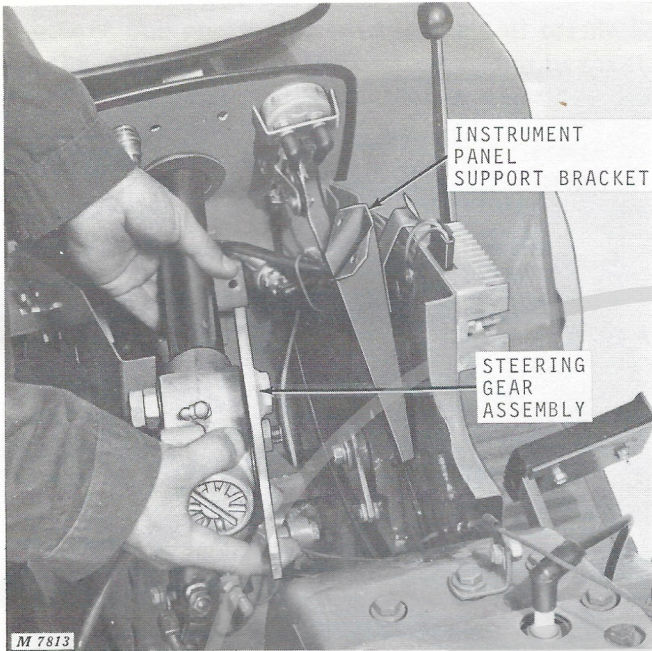
Figure 6A—Removing Steering Gear from Tractor
